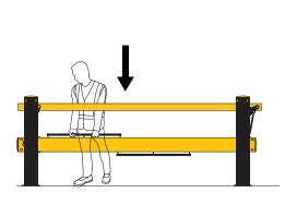
Lower the gate gently onto to the locator pin. Ensure that the gate is fully down and in its final resting position before you remove your hands.
