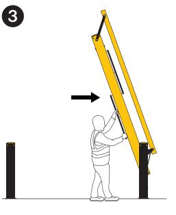
Continue to walk the gate to the hinge end. You will feel the gate gas strut take the weight of the gate and pull towards the vertical position.
