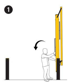
Before you start to lower the gate, please ensure that an area around the hinge end of the gate is clear of people and objects. Use your left hand to release the locking mechanism. Gently pull the gate towards you.
