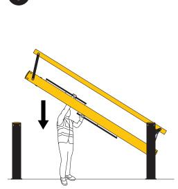
When the gate is at a comfortable descending height, move your right hand to the top handle. As the gate descends further, move your left hand to the top handle.
