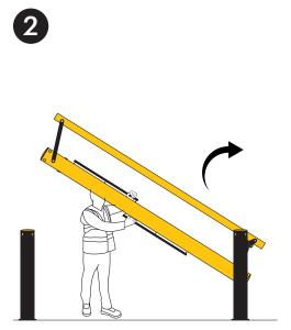
Slowly walk the gate towards the hinged end. When the height of the top handle comes out of reach and uncomfortable, use your right hand to grab the bottom handle.
