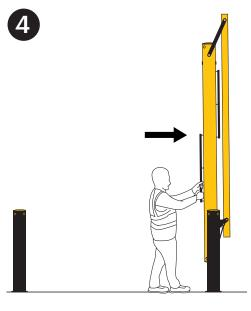
Gently ease the gate to its final resting position. You will hear and feel the locking mechanism click in to place. It is now safe to remove your hands off the gate.
